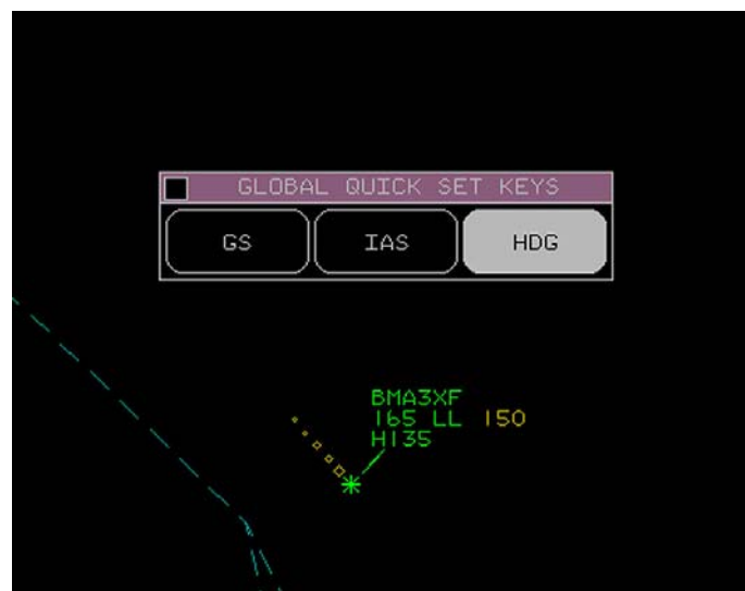
Fig 1: Mode S information in the Target Label.
