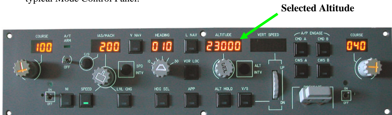
Fig 3: Mode Control Panel
