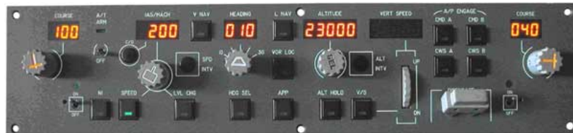
Fig 1: Typical Mode Control Panel showing selected altitude of 23000
